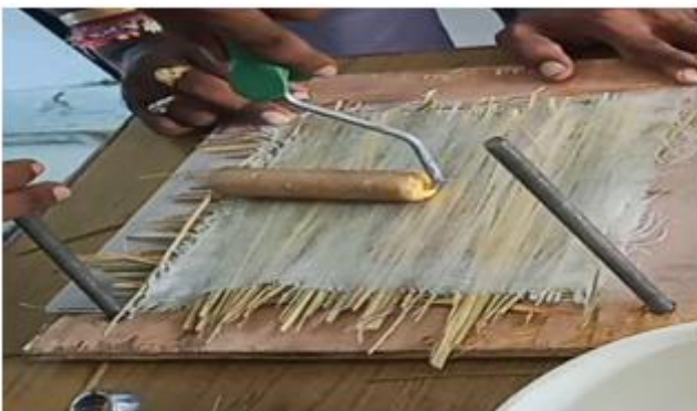
Figure:6. Hand layup method
