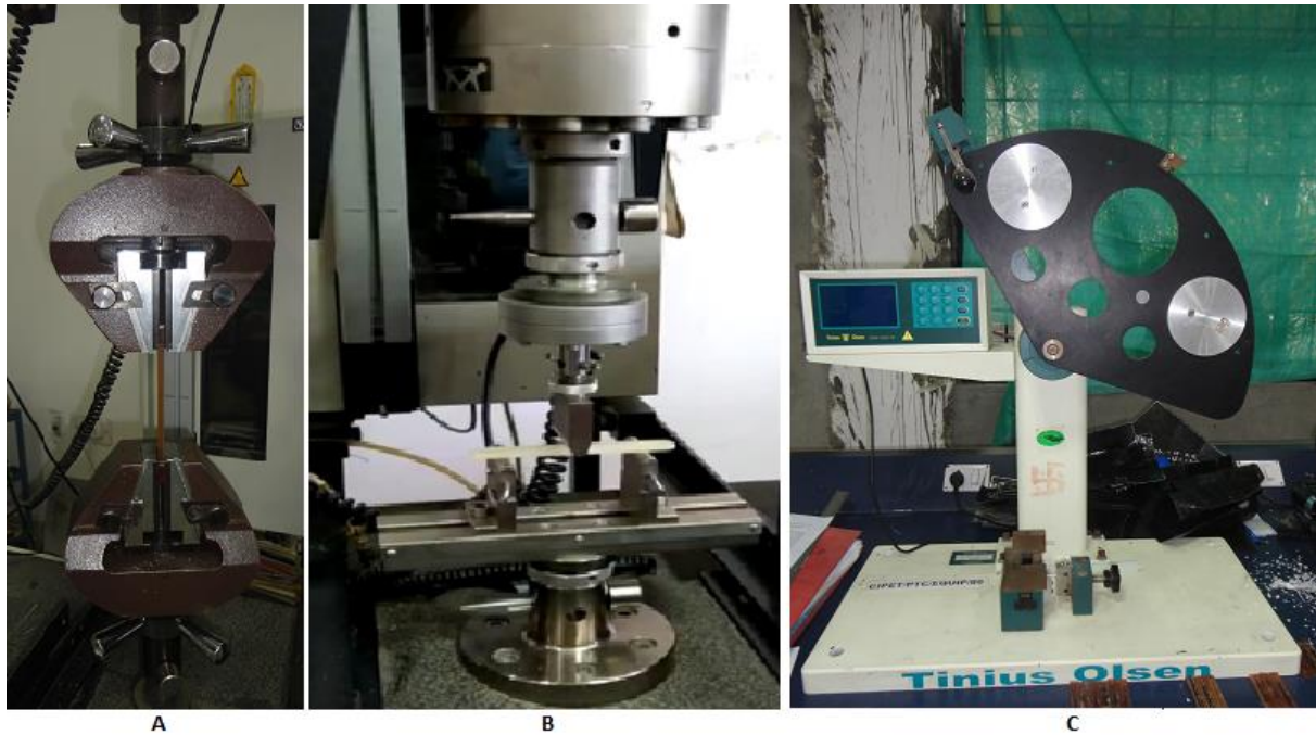
Figure 2: Setup for (A) Tensile (B) Flexural and (C) Impact tests
