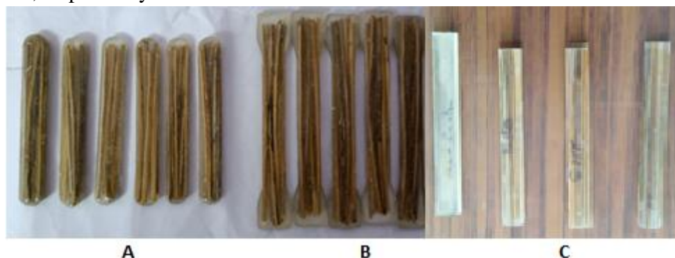
Figure 1: Specimens for (A) Flexural Test (B) Tensile Test (C) Izod Impact Test
