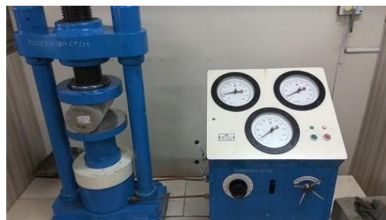
Fig.2 Split tensile testing
