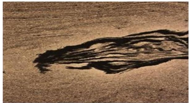
Fig (4) cross sectional area of the produced FSW showing Monel400 inside Carbon steel
