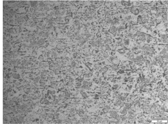
Fig(2) Microstructure of 1020
