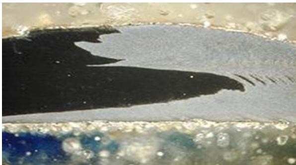
Fig (3) cross sectional area of the produced FSW showing the carbon steel inside Monel400
