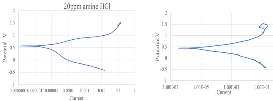
Fig 9 (a) cyclic potential of FSW specimen in 10% HCl      Fig 9 (b) cyclic potential of SMAW specimen in 10% HCl Specimens were submerged in 10% HCl for 30 days and then after removing the solution Monel400 showed redish metal and a new phenomenon was observed and this was denickelation and it's a kind of dealloying.
