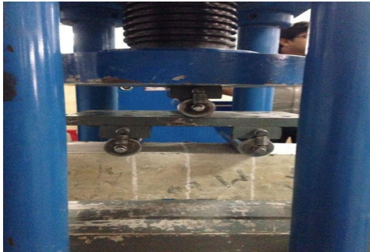
Fig. 4 Testing of fly ash & quarry dust concrete beam
