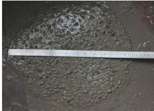
Fig.2 Sump flow test
