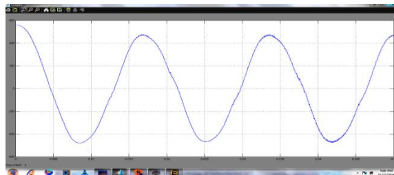
Fig.18. current flowing through hot wire 1 of distribution transformer 11
