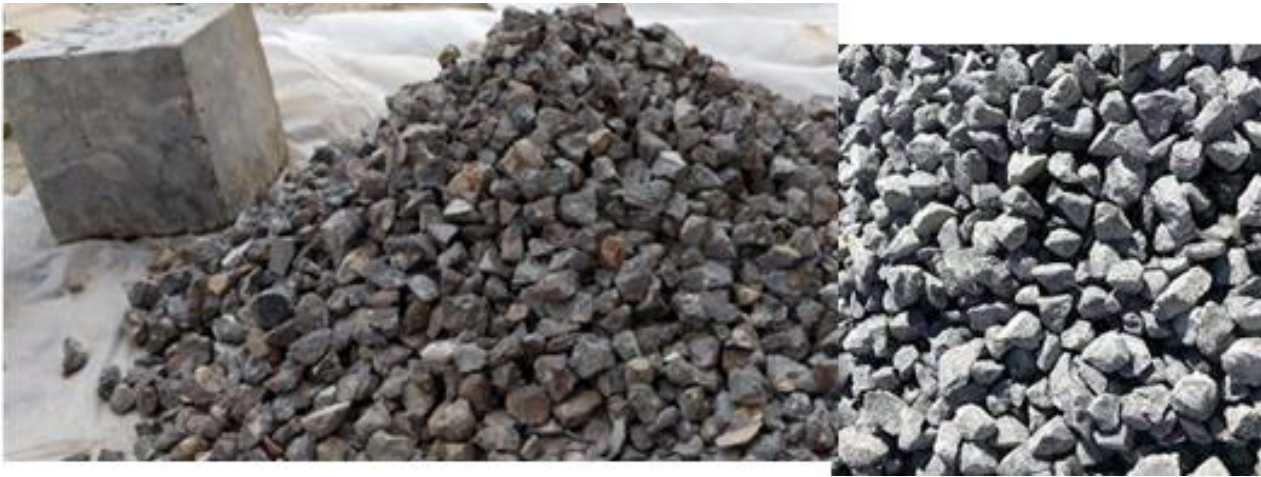
Figure 2: Recycled Concrete Aggregates (RCA)
