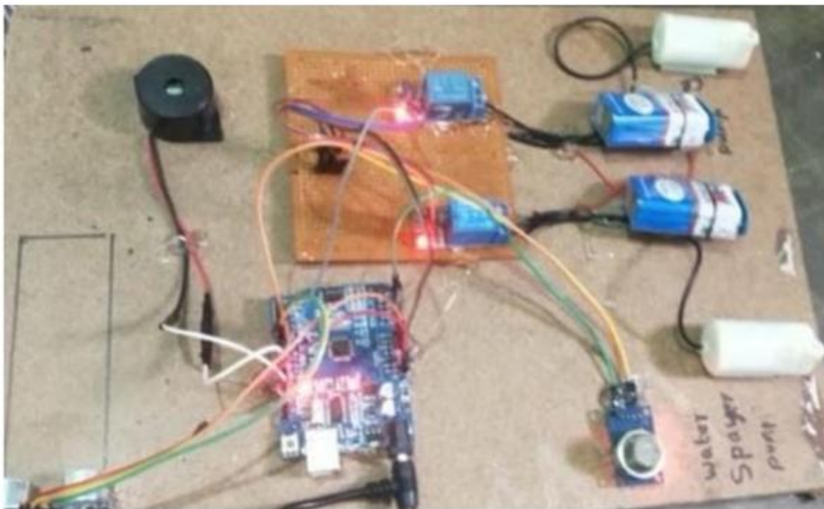
[IV] Water Head Sprinkler and Buzzer is activated when fire is detected
