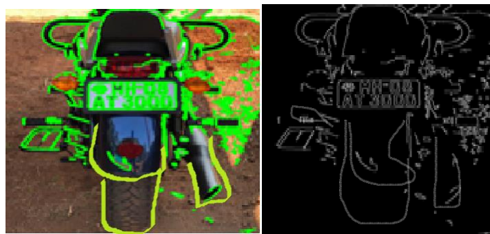
Fig. viii to show the finding edges of the grayscale image
