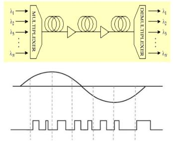
communication of information having data rate higher than 10 Gbit/s is achieved using a popular technique which is known as wavelength division multiplexing (WDM). Several signals with different wavelength are sent through the same optical fiber using this technique.
